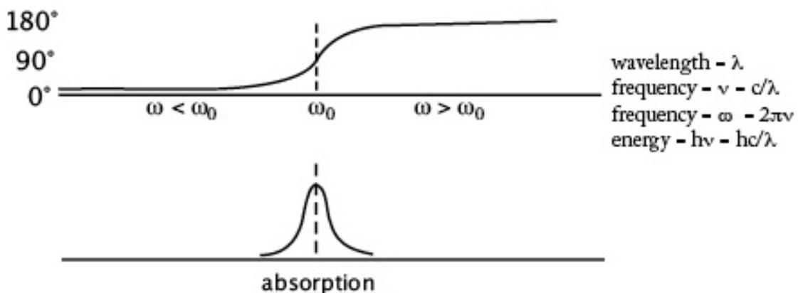
**DEMO:** plumb bob pendulum (variable frequency) driving pendulum Styrofoam ball oscillator (electron). Relative phase of plumb bob (driving wave of frequency  $\omega$ ) with ball pendulum (native frequency  $\omega_0$ )
